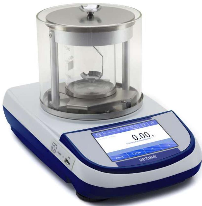
TS-iDens is a Balance for density calculation, in particular it is designed to easily determine the Density Index of a solid sample without need of any computer software or external database.
