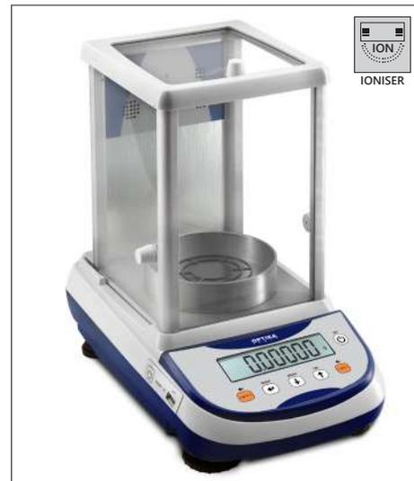
I-models equipped with integrated ioniser on the back of the balance. The ioniser has two way of operating: 2 minutes or continuously for max 8 hours.
